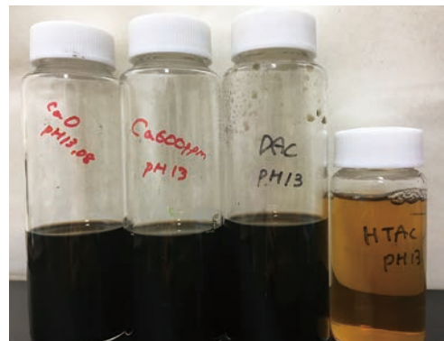
Fig. 27 Photographs of filtrates from Kuroboku-soil suspension at pH 13 including none, 600 ppm of Ca, 5.5 \times 10^{-5} \text{ mol/L} of DAC and 7.5 \times 10^{-4} \text{ mol/L} HTAC from the left
