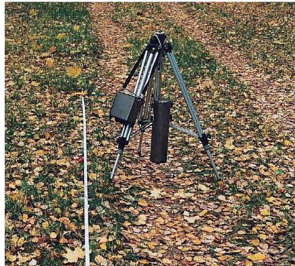
Fig. 4 A scintillation portable gamma-ray spectrometer mounted on a tripod
