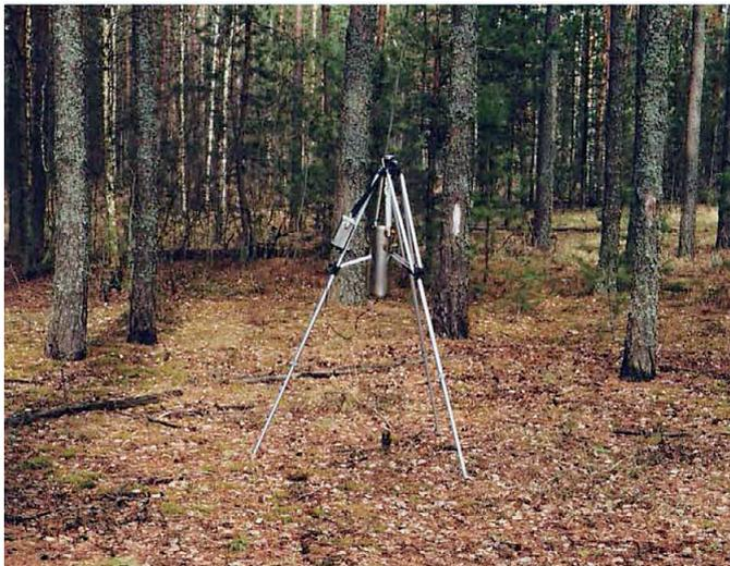
Fig. 3 A scintillation portable gamma-ray spectrometer mounted on a tripod
