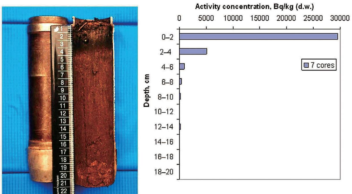
Fig. 13 Vertical distribution of activity concentration (dry weight) of <sup>137</sup>Cs at an untreated plot in Muravinka in 2002 (to the right) and a soil core sampled on the plot (to the left)
