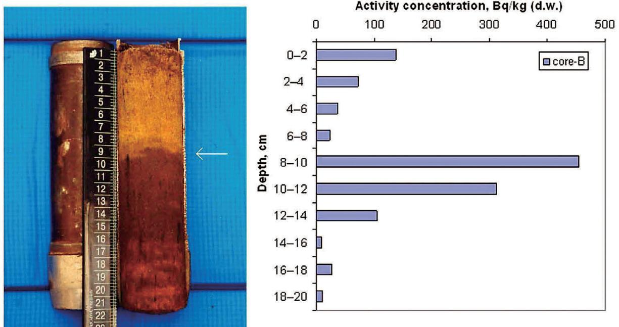
Fig. 12 Vertical distribution of the activity concentration of  $^{137}\text{Cs}$  (to the right) in a soil core (to the left) sampled on treated plot in Muravinka in 2002
