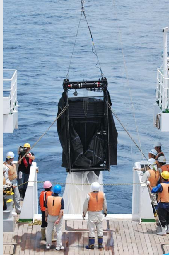
Sampling with a submersible pump
