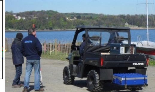
Vehicular 2s measurements – capable of locating radium sources at lateral distances of 1m and burial depths of 30cm
